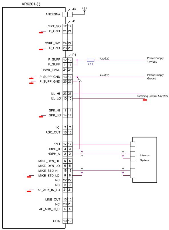
Figure 2-9 Typical Wiring for Aircrafts with Intercom System (unbalanced)
