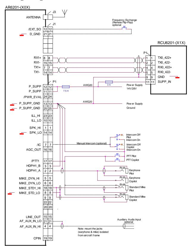
Figure 2-11 Typical Wiring for Twin Seater Aircrafts, Tandem
