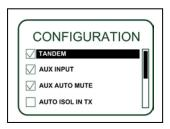
The CONFIGURATION page consists of 6 (max.7) selectable options. (refer to the Note under "AUX AUTO Mute" in the column on the right side) Use the "ROTARY ENCODER" to scroll up and down.
