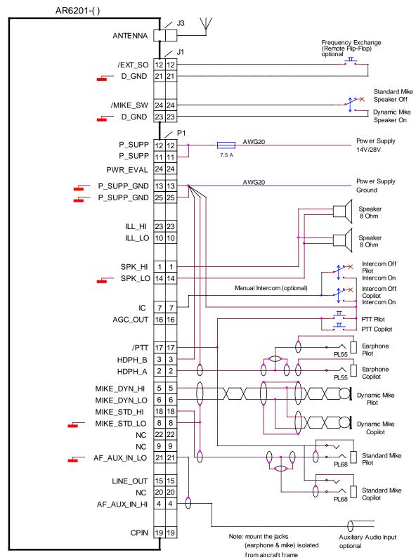
Figure 2-7 Typical Wiring for Twin Seater Motor Glider
