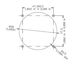
Figure 2-3 Drilling jig for back-panel mounting
