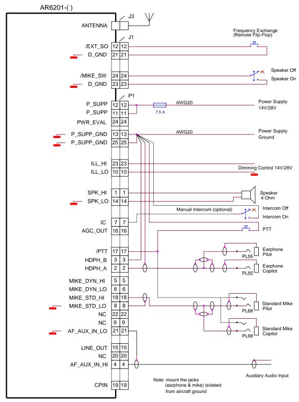
Figure 2-8 Typical Wiring for Standard Headsets in use
