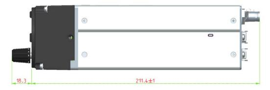
Figure 2-1 VHF transceiver side view
