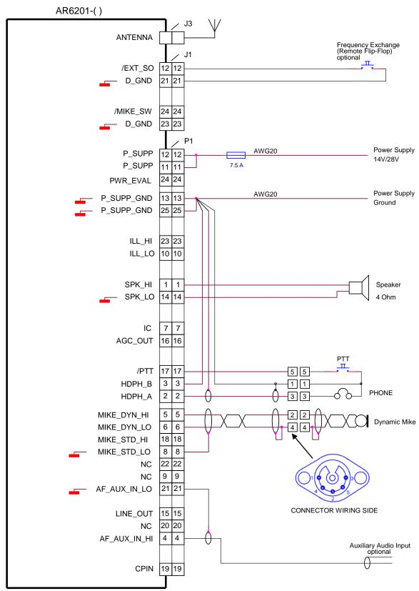
Figure 2-6 Typical Wiring for Single Seater Gliders (5-pol DIN Jack)
