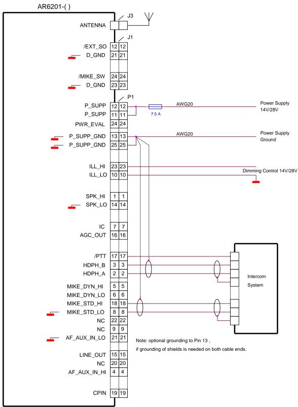
Figure 2-10 Typical Wiring for Aircrafts with Intercom System (balanced)
