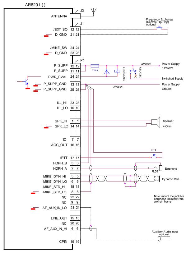
Figure 2-5 Typical Wiring for Single Seater Glider
