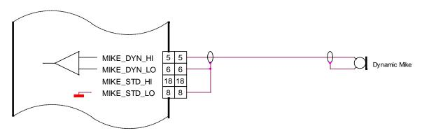
Figure 2-14 Modified Dynamic Microphone interwiring for AR6201
