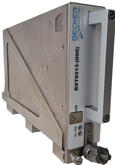
Transponder BXT6500 Series with backshell and mounting tray
