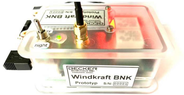
Illustration 2: Prototype for a on-demand night time marking system
