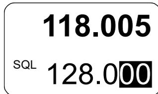
A short press of the "↕/SCN" key, exchanges active frequency to preset frequency and vice versa. If wanted, please press now the "STO" key to store the active frequency into the next vacant memory place of the user channels database.
