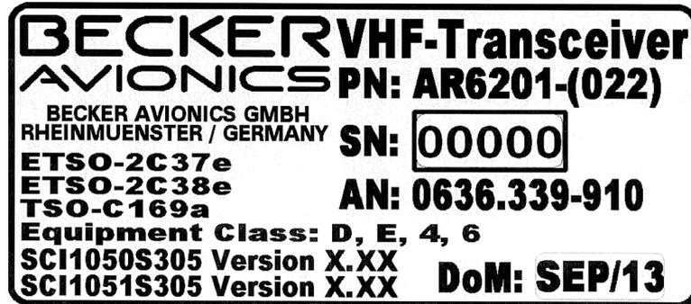
Figure 2-1: Type plate (example)
