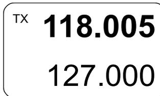
In transmit mode several user actions such as changing frequency selection mode or channel spacing mode, which are normally allowed in receive mode, are blocked. (As an exception in standard mode the "Preset" frequency may still be changeable, even during transmission).
