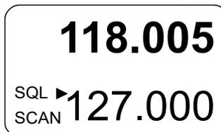
**Note:** Transmission always uses the active frequency, even if the monitored frequency is currently audible.
