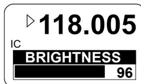
The panel brightness for display illumination and push buttons can be changed from 0 (illumination off) to 100 (maximum brightness) by turning the "ROTARY ENCODER".
