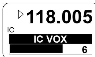
By means of the "ROTARY ENCODER" the intercom VOX threshold can be changed from -30 (most sensitive, even a very low microphone signal already triggers the VOX threshold for Intercom operation) to +10 (VOX is less sensitive and only high microphone signals trigger the VOX threshold for intercom operation).
