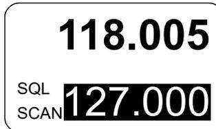
If selected in the configuration setup an audio notification "beep" tone becomes audible in addition to the blinking preset frequency to indicate the presence of an RX signal on the preset frequency.
