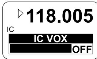
With VOX switched "OFF", activation of intercom operation using the external intercom switch (/IC discrete input) is still possible at any time. The VOX threshold level is not adjustable if VOX forced to be "OFF" (due to enabled speaker in current audio configuration).
