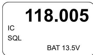
**Note:** The battery information is only displayed if BATTERY VOLTAGE in the configuration setup is selected.
