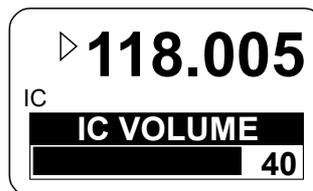
By means of the "ROTARY ENCODER", the intercom volume is changeable from zero to 46. The intercom volume setting affects the intercom audio and sidetone signal, routed to the headphone.
