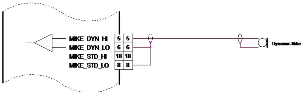
Figure 3-2: Modified Dynamic Microphone Wiring Interface for AR6201
