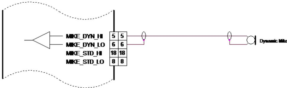
Figure 3-1: AR6201 with Wiring Interface for AR4201
